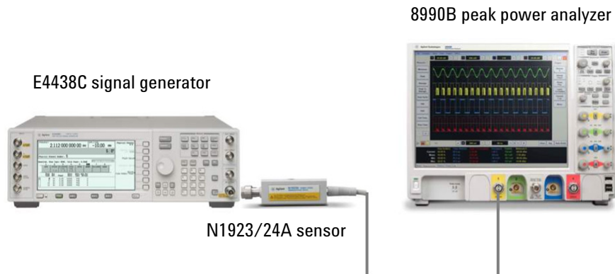
Figure 20-1 Test setup for the pulse characterization measurement
